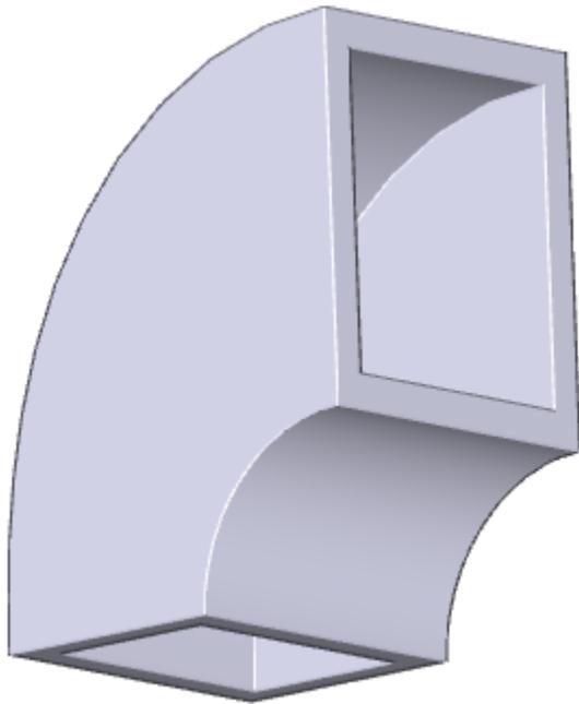
Example of solid coil, created by lofting and rotating profiles
